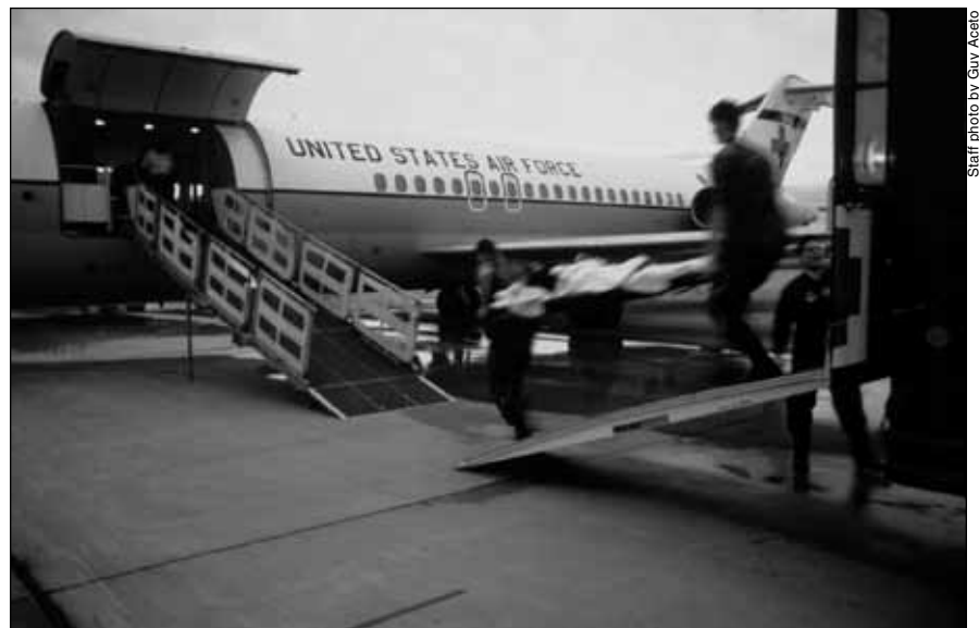
Long-distance air evacuation from Vietnam to the Philippines, Japan, and the US spurred USAF to acquire specially built C-9 Nightingale hospital aircraft. The C-9 can carry 40 litter patients with five medical personnel.
